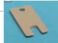
Mini anion exchange column opener is used to remove the lower stopper of the column by pushing the opener between the white stopper and the column bottom.
