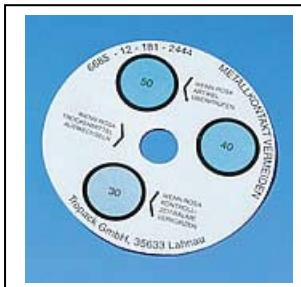
Card with spots printed with cobalt (II) chloride solution varying in concentration. The numbers inside the moisture sensitive spots indicate the relative humidity with a visible colour change from blue to pink.
