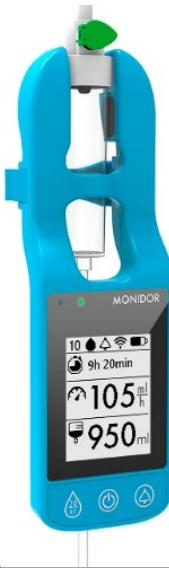
The electronic drop counter gives direct visibility to the ongoing gravity intravenous therapy. The device is easily clipped into common drip sets and the display clearly shows infusion speed, total volume, time and targets related to volume and speed. The Drop factor (number of drops / ml) is fixed at 20 drops / ml, the device can therefore NOT be used with burettes (60 drops/ml) and is no longer included in the nutrition IPD module.
