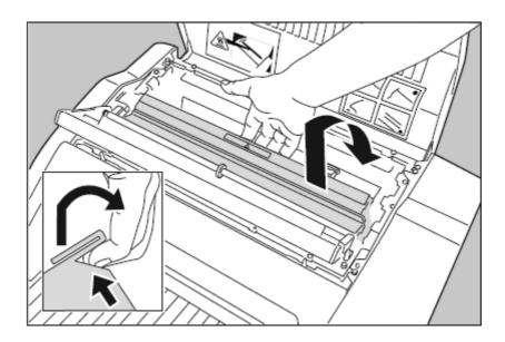
9. Locate and check on sight the print head resistor line.
