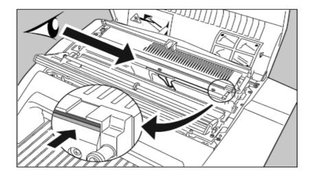
**WARNING:** Be careful not to touch the print head resistor line with your fingers. The print head unit can be warm.
