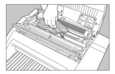
**WARNING:** <u>Do not apply any pressure on the print head</u> because this pressure may cause damage on the interconnections underneath the print head.
