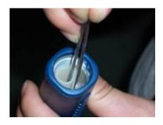
7. Create a circuit between the round metallic contact on the bottom of the compartment and the compartment wall for approximately 2-5 seconds.
