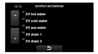
The first 5 outputs are displayed on this screen. To view the remaining outputs and scroll through the screen use the and keys. To force the outputs just press the required output.
