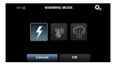
Press the key on the type of heating screen to select electric heating (resistors).
