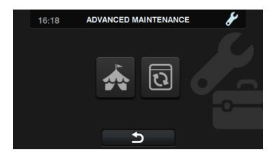
In exhibition mode, the washing machine ignores all the errors which are triggered, and runs a short demo programme.
