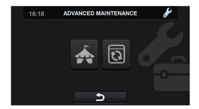
If this mode is active, any programme can be run indefinitely, that is, when the programme ends, the door is unlocked, the buzzer is sounded to open the door, but the programme will automatically start again, locking the door and running the configured phases.
