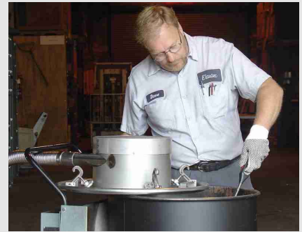
3 IGNITE LOAD - TURN ON MINIMUM AIR
