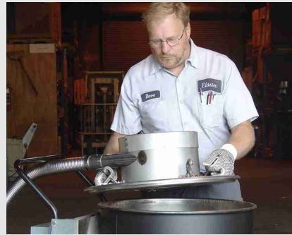
2 ATTACH AIR HOSE – REST LID ON DRUM
