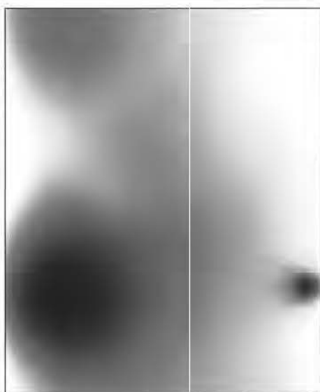
Fig 1.4 Example of film-fogging caused by LED of cell phone in a darkroom.
