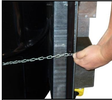
29. Wrap chain around barrel. Pull tight to remove any slack and attach to second hook.
