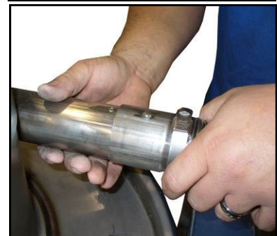
33. Slide flex hose over snap button on 2-inch inlet on drum lid.
