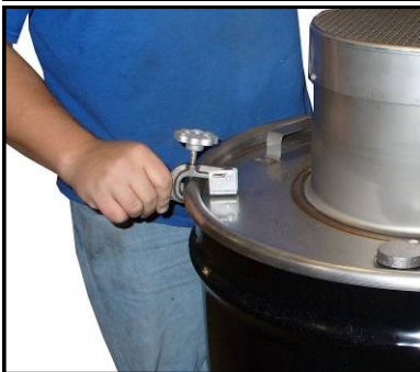
31. Rotate clamps into position and tighten by turning knob.
