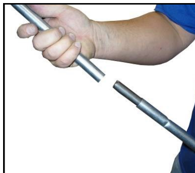
35. Assemble stir rod by inserting upset end over straight end and push together.
