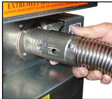
32. Slide flex hose over snap button on 2-inch outlet on plenum.
