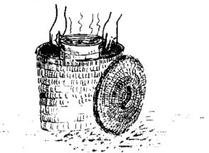
A good idea is to use a straw basket equipped with a lid and filled with insulating material such as dry hay, straw, dry leaves, wood shavings or crumpled newspaper. A nest is formed in this material to accommodate the pot. To avoid pieces of insulating material falling into the food, the nest may be lined with a piece of rag or cloth tucked in at the sides of the box.
